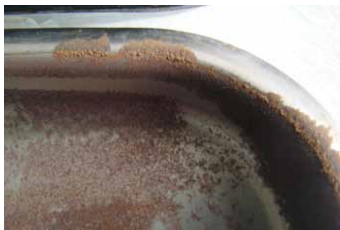
Randcorrosie schaalhelft expansievat. © Materials Consult.
